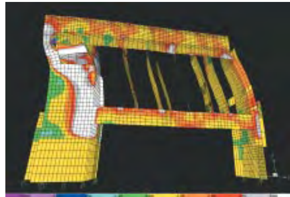
The baptistery fin walls and beams were coupled to form a Vierendeel truss, opposite and above , that spans the width of the nave and provides lateral stability to the rear of the cathedral. The truss concept was developed by Nabih Youssef & Associates to provide greater visual and auditory transparency.
